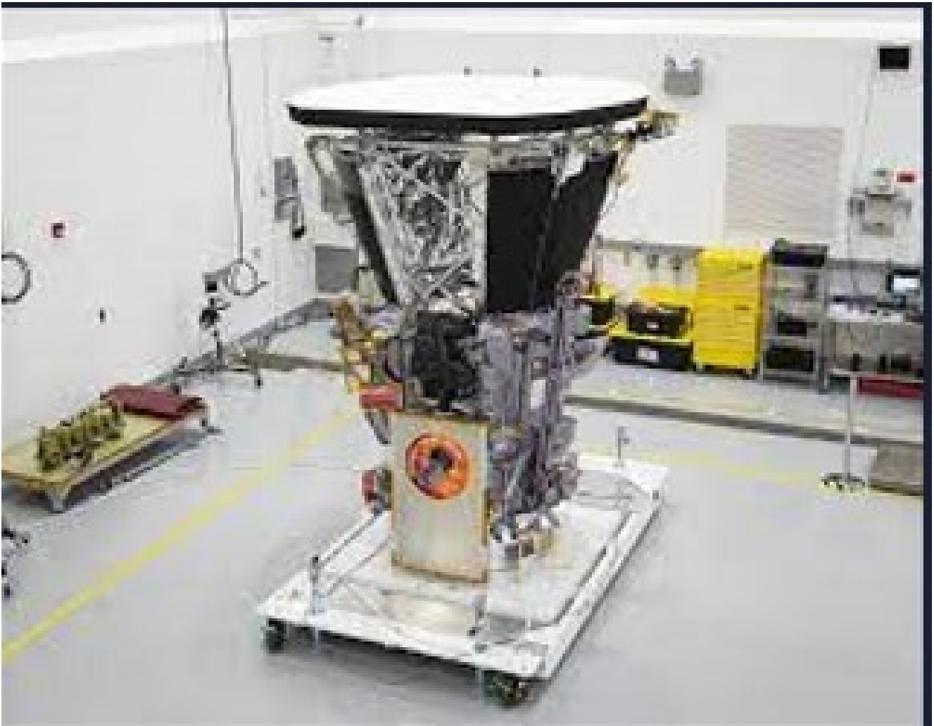
The Parker Solar Probe with its heat shield, solar array, and Kevlar-composed Micrometeorite Protection System under testing [Image Credits: NASA]
